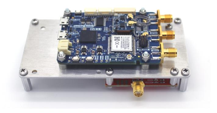
The ZED-F9P can be powered using the EVB-2 +3.3V output. Either serial 0 or serial 1 can be used to communicate with the ZED-F9P. See the EVB-2 H7 pinout for details.
