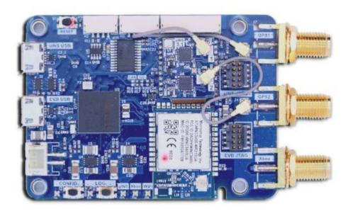
The Inertial Sense EVB-2 is a development board which contains the Inertial Sense  $\mu$ INS,  $\mu$ AHRS, or  $\mu$ IMU module. The EVB-2 builds on the foundation established by the EVB-1, but adds new features including:
