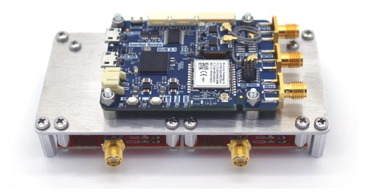
Two ZED-F9 units can be used to provide either or both multi-band RTK compassing and RTK positioning for the INS solution. The ZED-F9Ps can be powered using the EVB-2 +3.3V output. Serial port 0 and 1 must both be used to communicate with the ZED-F9P.
