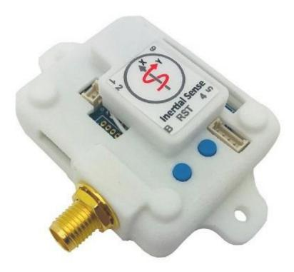
The Inertial Sense EVB1.x is a development board which contains the Inertial Sense  $\mu$ INS,  $\mu$ AHRS, or  $\mu$ IMU module. The EVB1.x functions as a breakout and communications board with the following features:
