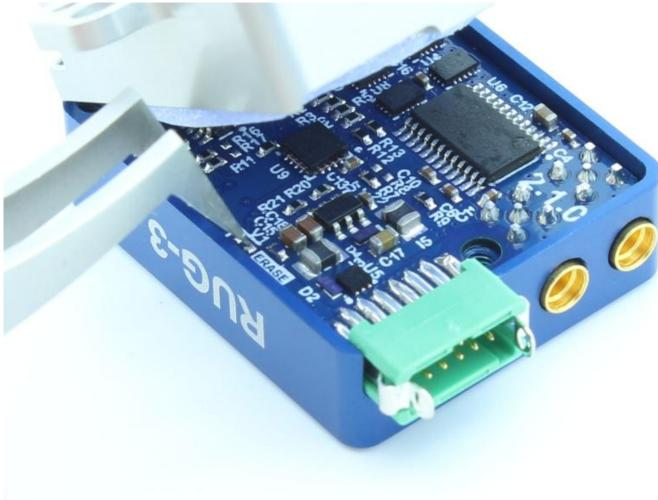
Short "ERASE" pads together and reset to chip erase.
