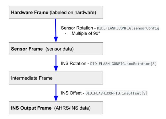
NOTE: The *Hardware Frame* and *Sensor Frame* are equivalent when the sensor rotation in <code>DID\_FLASH\_CONFIG.sensorConfig</code> is zero. The *Sensor Frame* and *INS output Frame* are equivalent when the <code>DID\_FLASH\_CONFIG.insRotation</code> and <code>DID\_FLASH\_CONFIG.insOffset</code> are zero.
