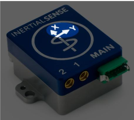
The IMX follows the right rule for XYZ axis relative direction and angular rotation.
