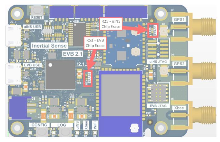
Short R25 pads together to chip erase uINS. Short R53 pads together to chip erase EVB-2.
