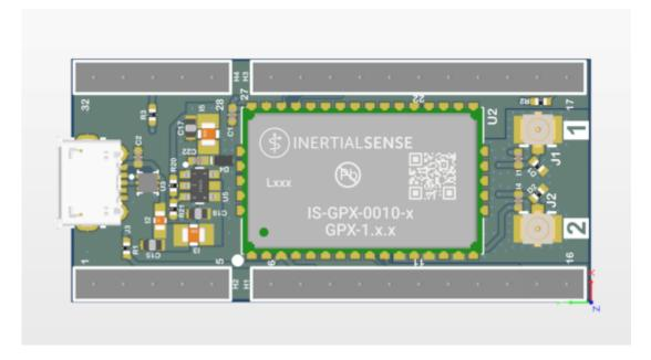
The Inertial Sense IK-1 is a breakout evaluation board for either the IMX-5 or GPX-1 multi-frequency GNSS receiver.
