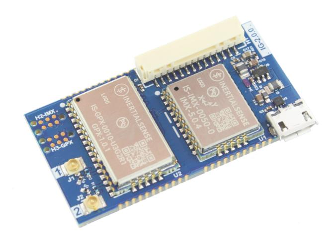
The Inertial Sense IG-2 is a PCB module with IMX-5 and GPX-1 multi-frequency GNSS receiver.
