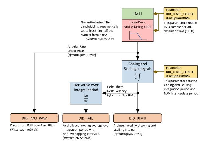
The preintegrated IMU (PIMU) a.k.a. Coning and Sculling (delta theta, delta velocity) integrals serve as an anti-aliased moving average of the IMU value. The DID\_IMU is the derivative of the DID\_PIMU value over a single integration period.
