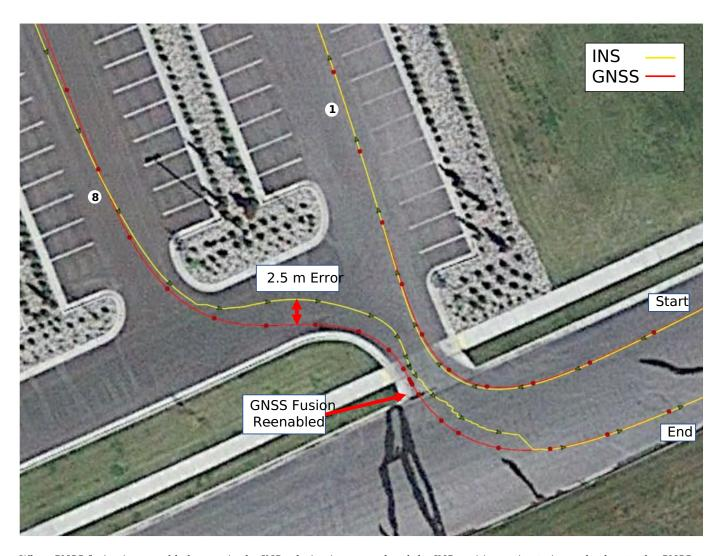
When GNSS fusion is re-enabled, error in the INS solution is removed and the INS position estimate jumps back onto the GNSS position. There is 2.5m of error between the dead reckoning position and the GNSS position.
