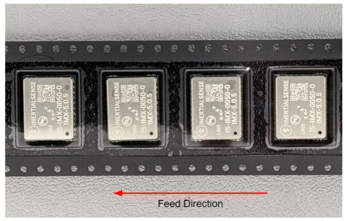
The feed direction to the pick and place pick-up is shown by the orientation of the IMX-5 pin 1 location. With pin 1 location on the bottom of the tape, the feed direction into the pick and place pick-up is from the reel (located to the right of the figure) towards the left.
