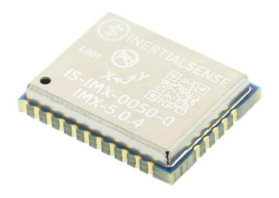
The IMX-5<sup>™</sup> is a 10-DOF sensor module consisting of a tactical grade Inertial Measurement Unit (IMU), magnetometer, and barometer. Output includes angular rate, linear acceleration, magnetic vector, and barometric pressure and altitude. IMU calibration consists of bias, scale factor, cross-axis alignment, and temperature compensation. The IMX-5 includes Attitude
