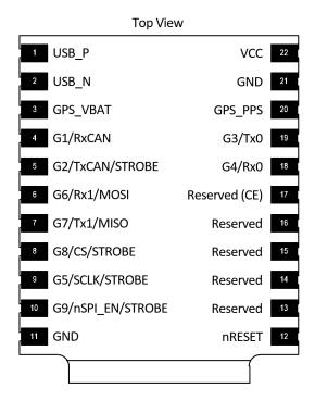
STROBE pins on the µIMU, µAHRS, and µINS Module - Top View
