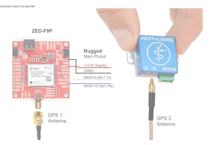
A +3.3V or +5V supply is needed to power the ZED-F9P when using the Rugged-1 IMX. A USB +5V supply can be used if available. The Rugged-1 must be configured for Serial Port 1 TTL voltage. See hardware configuration for Rugged v1.0 or Rugged v1.1 for details.
