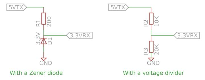
These circuits are beneficial because of their simplicity. An active, powered level shifter may also be used and necessary.
