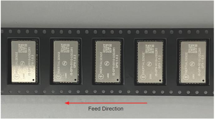
The feed direction to the pick and place pick-up is shown by the orientation of the GPX-1 pin 1 location. With pin 1 location on the bottom of the tape, the feed direction into the pick and place pick-up is from the reel (located to the right of the figure) towards the left.
