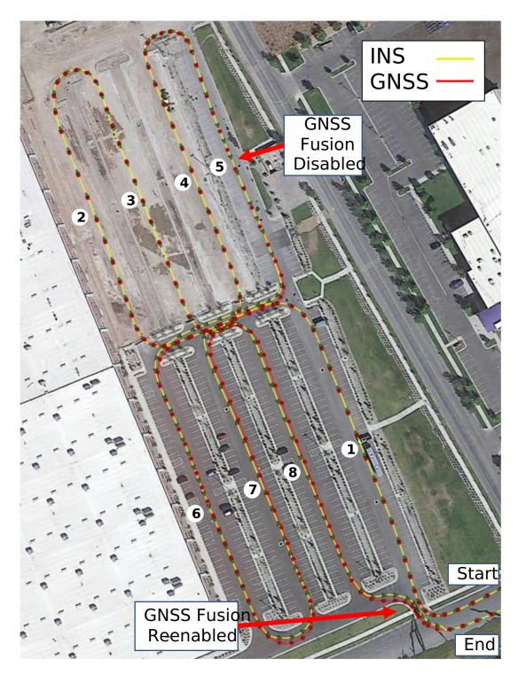
In the drive the car starts and ends the drive at the bottom right corner of the image. The numbered path segments show the order of travel. GPS fusion was disabled in the middle of path segment 5.
