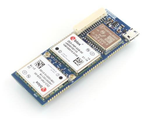
$The \ Inertial \ Sense \ IG-1 \ is \ a \ PCB \ module \ with \ IMX-5 \ and \ dual \ ublox \ ZED-F9P \ multi-frequency \ GNSS \ receivers.$
