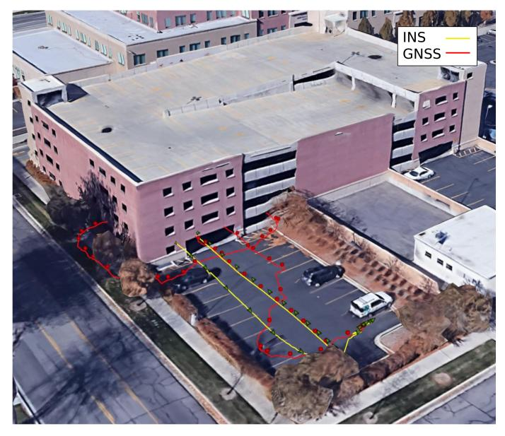
Here we see outside parking lot where the test vehicle started and ended. GNSS fix was lost upon entry of the garage and regained several seconds after exiting the garage.
