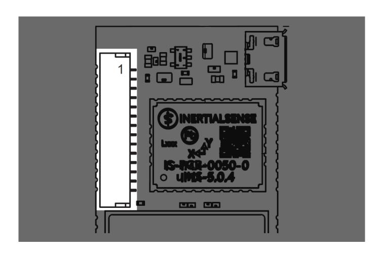
The IG-2 module and IG-2 header H1 have the same pinout assignment for pins 1-14. Because H1 only has 14 pins, pins 15 and above listed in the following table are only on the IG-2 module.
